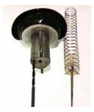
The slide is on the left, with the diaphragm above. The drill bit indicates the vacuum drilling that you may wish to consider enlarging. On the right is the spring, with needle "spider" and tapered needle. When assembled, the spring, needle carrier and needle sit inside the slide, with the needle sticking through the centre hole in the bottom of the slide.
