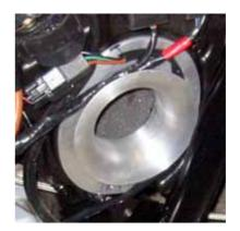
To take advantage of the improved airflow we increased the main jet size from 110 to 118 and put 2 shims under the needle. A visit to the Dynamometer at local racing team (Crescent Suzuki UK) resulting in the technician suggesting that another shim would be a good idea. So with 3 shims I thought it was going well. **Wrong!** The technician was used to working with fuel maps and doing everything with a computer: the bike still didn't run as I felt it should.
